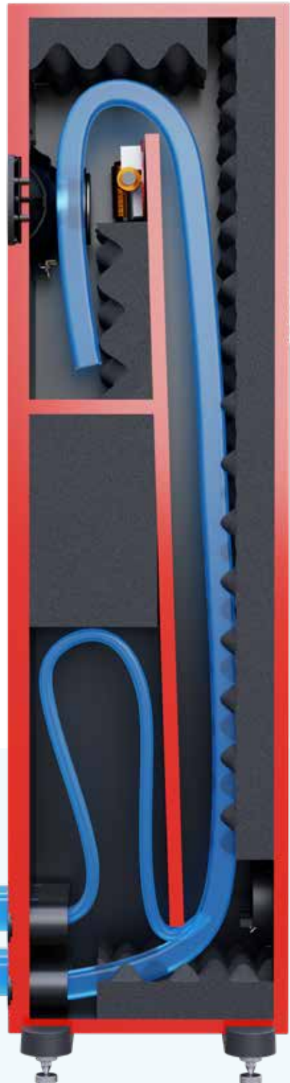
prodigy5 showing ATL in cross-section with Laminair vent
