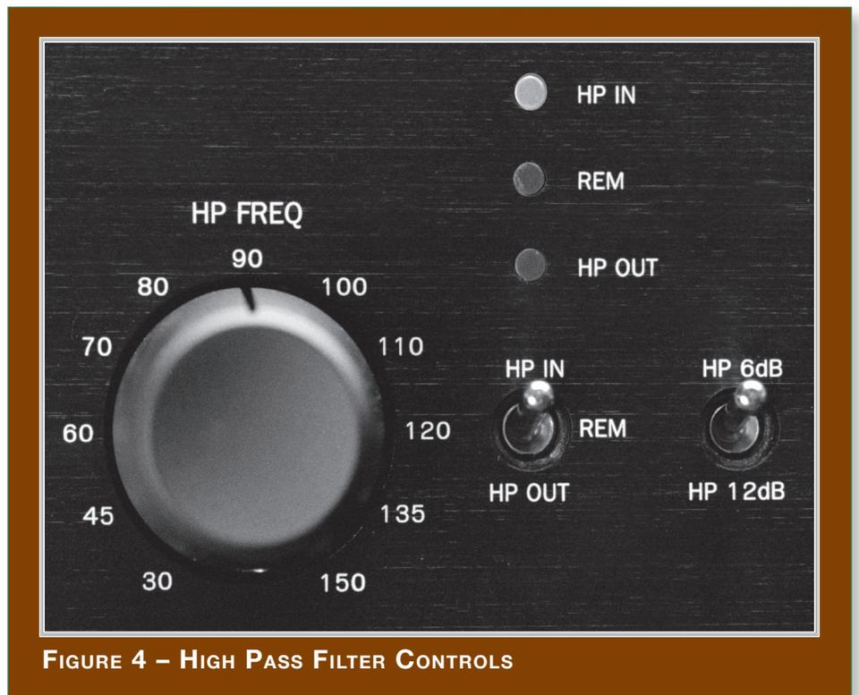
FIGURE 4 – HIGH PASS FILTER CONTROLS
