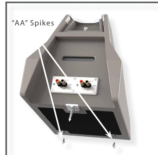
“AA” spikes are always installed in the front two positions (the threaded holes located near the bottom front of the enclosure). The spike-type is stamped in the round top of the spike. The two “AA” spikes screw into the Upper Array. The spikes should be screwed in all the way, until they are hand tight. Do not over tighten spikes.
