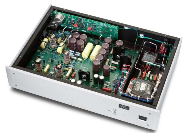
The TP-2.5*i* shares the same cosmetics as the TL-2.5*i* preamplifier with aluminum top and thick sides that mount to a well-braced chassis, offering better rigidity and bracing, and also a non-ferrous loop around the audio circuit.
