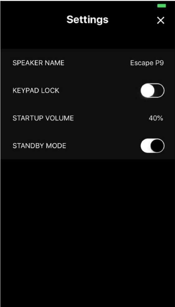
**Adjust startup volume. Change settings between 10% and 50% and press Confirm button**
