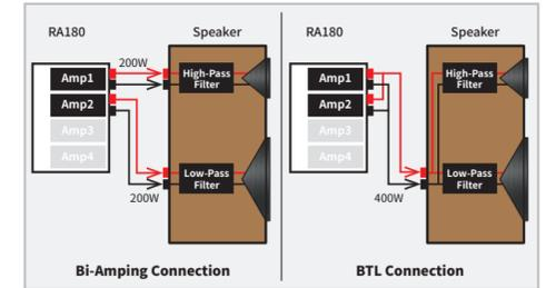
Connection to the speaker: Bi-Amping connection / BTL connection
