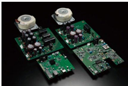
Esoteric Network Engine G4 (left), digital audio circuit (right), and dedicated large linear power supplies
