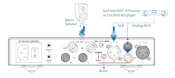
1. Toggle the Stereo/Mono switch to MONO.
