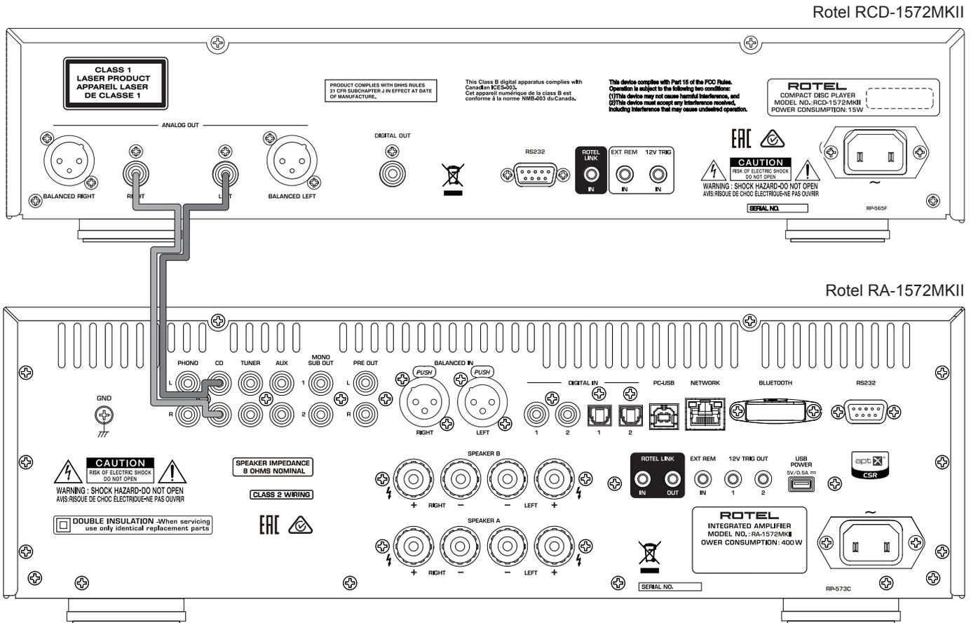
Figure 4 : **Balanced Outputs Connection**
