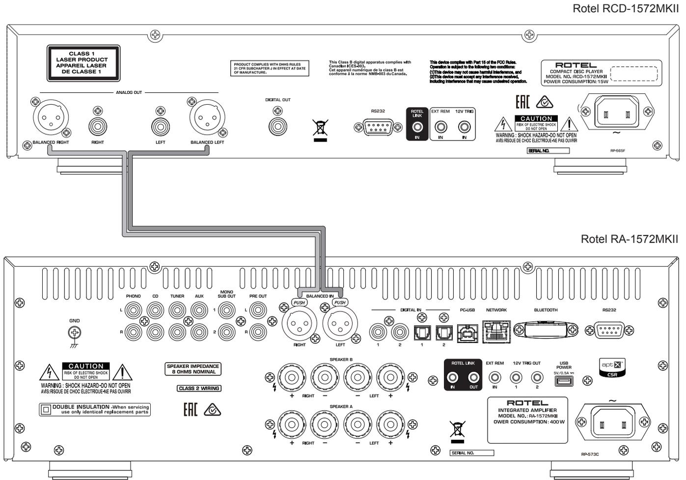
Figure 5 : Digital Output Connection
