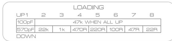
For all individual mini switches, when UP, the corresponding loading is OFF. When DOWN, the corresponding loading is ON.
