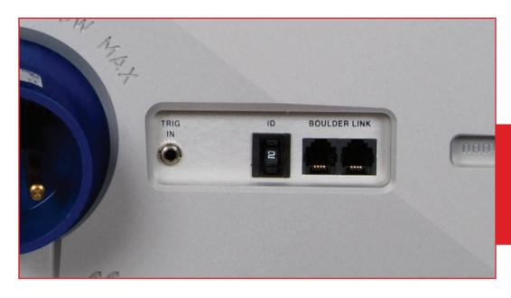
Boulder Link is a means of interconnecting most of Boulder products so that their microprocessors can talk to each other, pass important information, and issue commands. Among the key features, Boulder Link allows sequential initiation of power amplifiers' and other products. Boulder power amplifiers can send messages to Boulder preamplifiers which are then shown on its display.
