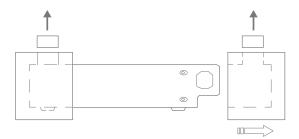
Open the box from the top and remove the accessories from the foam end caps. You may now proceed to lift the unit from the box, Once the unit is removed you can proceed with the removal of the foam end caps. These caps are designed to fit on the front and back of the unit for maximum protection. Retain the packaging for future transportation of this unit.
